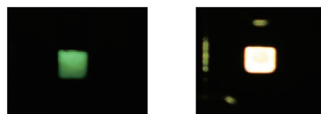
Figure 2. Emissions from ITO / m -MTDATA / PBD / LiF / Al device at 6 V (left) and 15 V (right).
