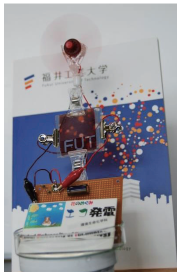
Fig.9 DSSC with electric double-layer capacitor.
