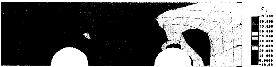
(c) \sigma_1 , MODEL-F ( t_s=9\text{mm} , T=8100\text{ kg} )
