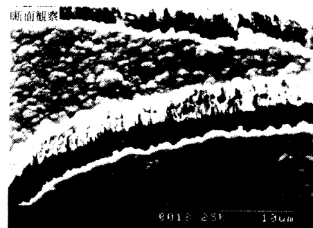
Fig.8 SEM photograph of ruptured Zn-Ni alloy film showing columnar structure.
