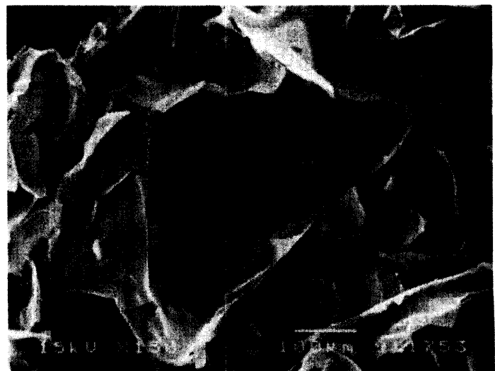
Fig.10 Scanning electron microphotograph of PU's containing 10% acetone.
