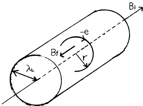
$$\begin{aligned} B_f L &= \mu n e r \left( \frac{e B_0}{m} \right) L \Lambda_L \\ \therefore B_f &= \frac{\mu n e^2}{m} r \Lambda_L B_0 \\ &= B_0 \frac{r}{\Lambda_L} \end{aligned} \quad (4.3)$$
