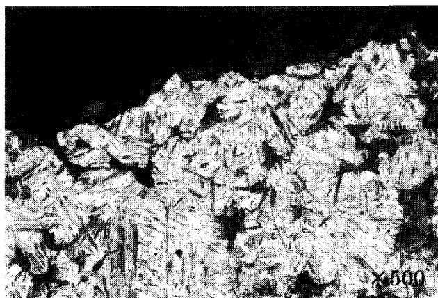
Fig. 10 Micro structure of sintered steel (PA-B)
