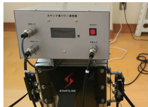
Fig. 1 Measurement device of kayak paddling power
