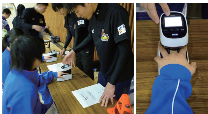
Fig.2 Noninvasive monitoring of hemoglobin concentration
