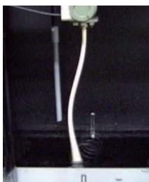
Fig. 2 Photograph of a self-excited pipe vibration
