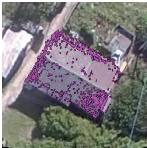
Fig.9 Resultant image with detection of damaged regions.
