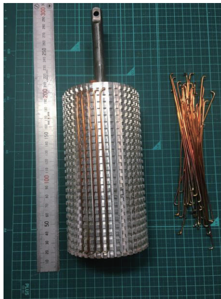
Fig.5 Heat storage material added on surface of displacer piston
