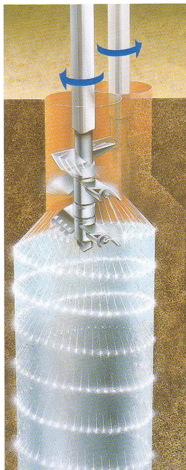
Fig.1.8 Schematic Diagram of JACSMAN Method
