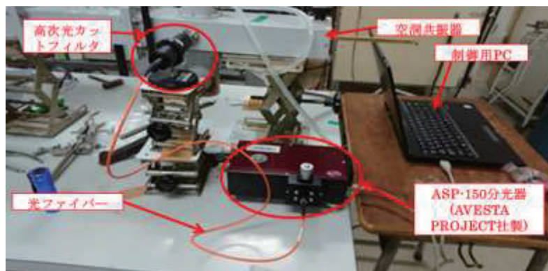
Fig. 3 Plasma spectroscopy measurement apparatus
