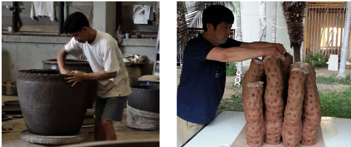
Figure 3.6 Hand-building method, Left- The Tao Hong Tai factory's craftsman making huge water jar by coil-pinch method, Thailand, Right- Sam Chill Park, Korean ceramic artist, shaping his organic form sculpture
