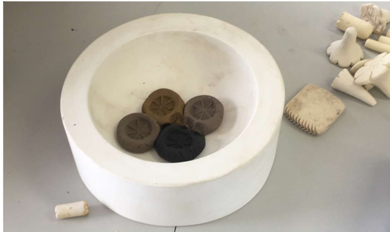
Figure 4.11 Piece of clay were press into the mold by stamp tools
