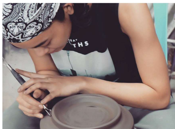
Figure 3.10 The author is making clay prototype of bowl on the wheel before the mold making process.
