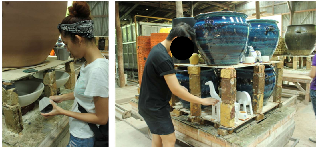
Figure 3.4 The gas kiln section of Tao Hong Tai Ceramics Factory, Thailand, Left-preparing products before loading in the kiln Right-loading out finished products
