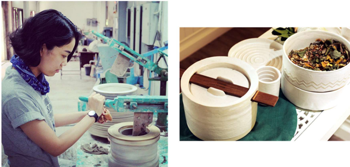
Figure 3.12 The author with Jigger-Jolley method, Left-Jolley method operation works with rotate plaster mold and shaping blade, Right- The Thai medicine tolls collection of the author made by Jigger-Jolley method
