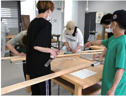
Fig.7 Draw a line at the position to be processed
