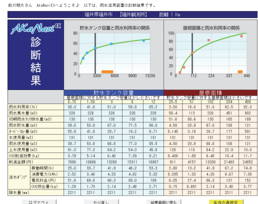
Fig. 10 Diagnosis test display of rainwater harvesting system.
