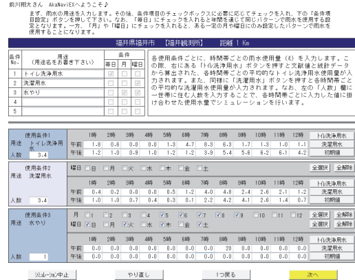
Fig. 8 Setting display of water consumption for rainwater harvesting system operation simulation.
