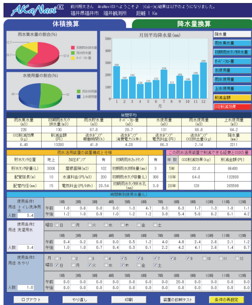
Fig. 9 Result display of rainwater harvesting system operation simulation.
