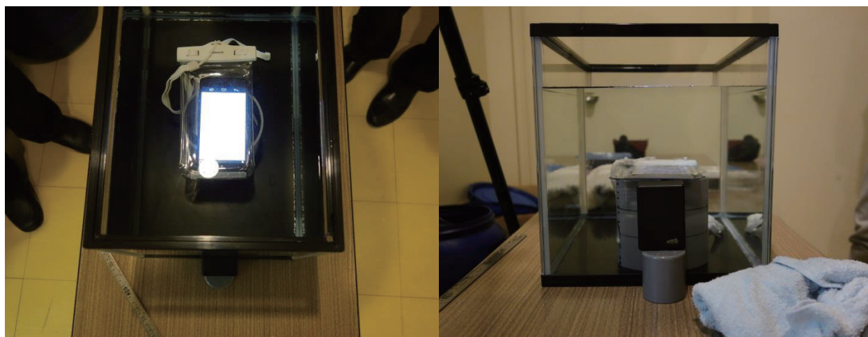
Fig. 6 Images in the experiment for detecting radio-field intensity in a water tank. A view from above (left) and that at the beacon-module side (right).
