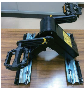
Fig. 1 Pedaling Electrical Generator
