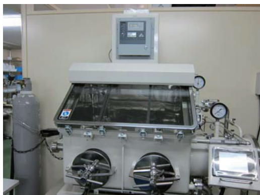
Fig.1 Glovebox used for the immersion test and contact test.
