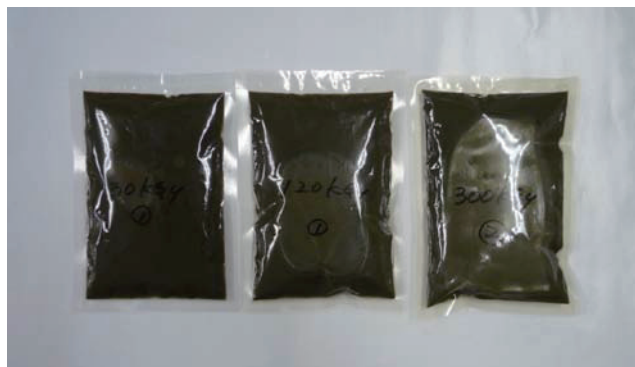
Fig. 1 Waste activated sludge after electron irradiation. 30, 120 and 300 kGy from the left.
