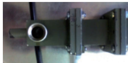
Fig.3 Scheme of the microwave resonant cavity
