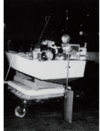
Fig. 2 Ship model with oscillating fin propulsion device
